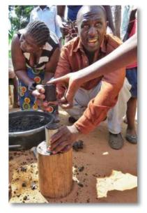
5) Push the cylinder down onto the top of the wood block. The cylinder will stay in place and push a briquette out the top.
