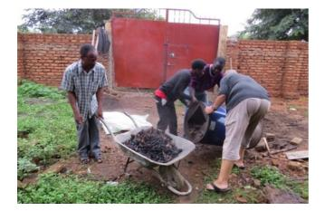
15) Once the drum has cooled, its contents can be emptied and the pyrolyzed maize cobs (now turned to real charcoal) separated from any cobs that have not completed the carbonising process.
