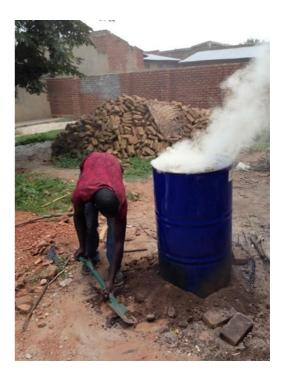
13) Finally, to completely seal the drum, Earth must be packed around the top and the bottom.
