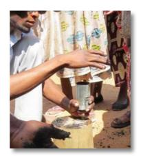
4) Lift the cylinder out of the hole in the wood block and rest the end of the bottom piston on the top of the wood block.
