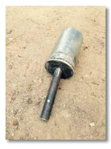
3) Place the long piston in the top of the cylinder and hit the rod 2 - 3 times with a hammer, a piece of wood or a stone.
