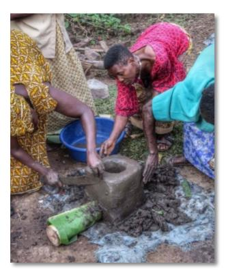
10) Remove the top pole, and then the leaf that was wrapped around it. The metal bars will remain in place at the bottom of the hole and the clay can be cleaned away from them later. Shape the top of the pile of mud with a knife to make it flat.
