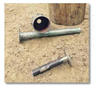
The **shorter** rod (piston) fits **into** the cylinder with the rod through the hole in the circular plate at the bottom of the cylinder.
