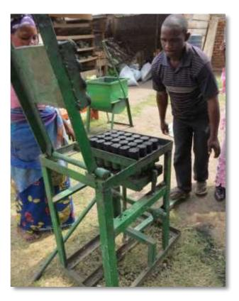
For larger scale briquette production, the steelcylinder style press can be incorporated into a multi-briquette press that will produce up to 24 briquettes in each pressing.
