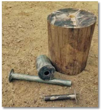
The timber block must have a hole in the top that is wide enough and deep enough to allow the **short** metal piston to be dropped into it once it is inside the steel cylinder.
