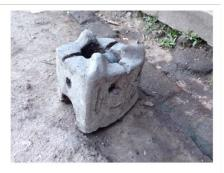
Rocket stoves work by making sure that all the heat goes to the pot and is not wasted around the fire.
