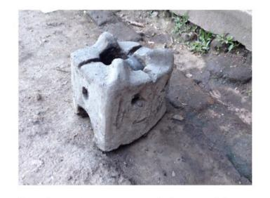
Rocket stoves work by making sure that all the heat goes to the pot and is not wasted around the fire.
