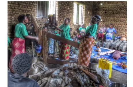
Finally the Fuel Briquettes are very carefully removed from their moulds and left somewhere safe to dry for 3-4 days. The Briquettes have truly become Fuel From The Fields.
